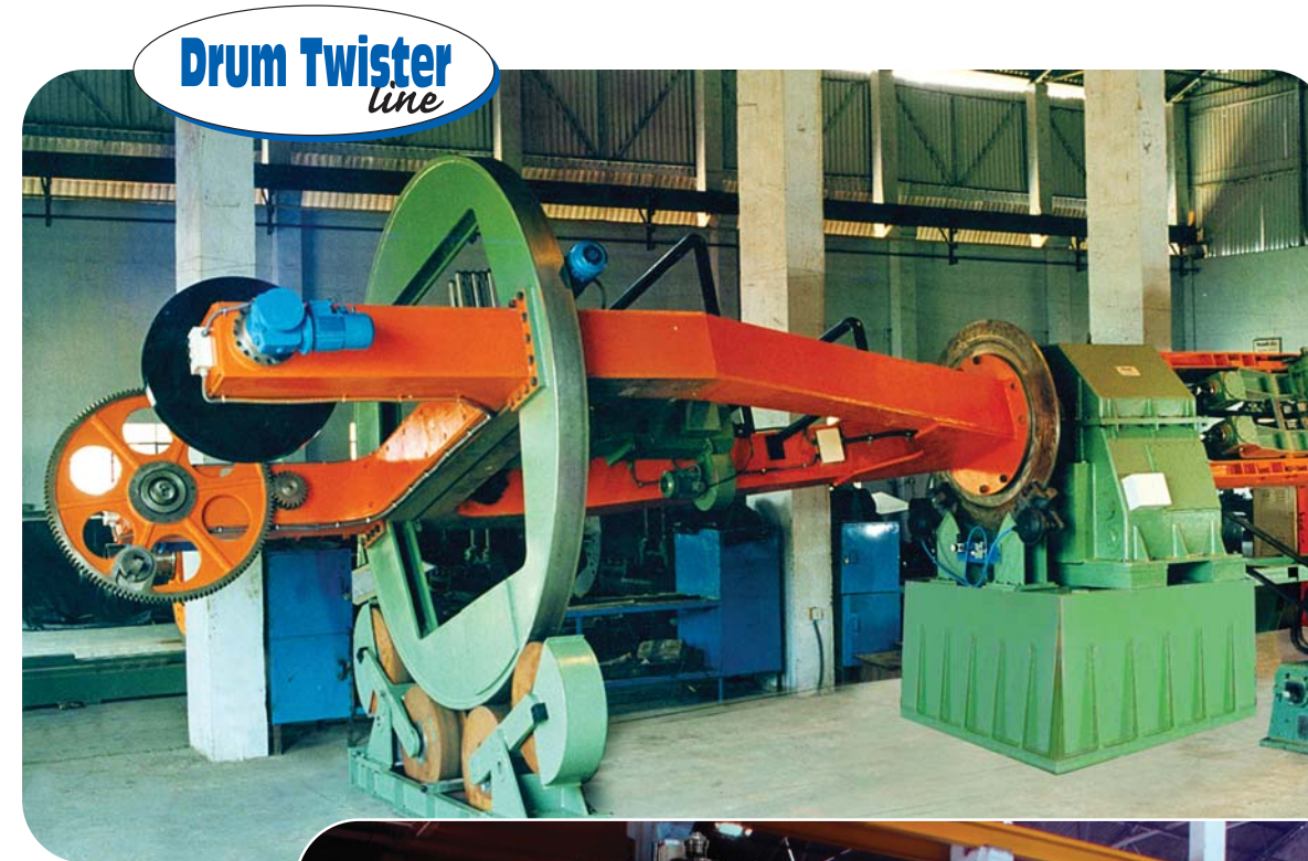
Under Roller Type Take Up Dia : 1600 ~ 3000 mm
